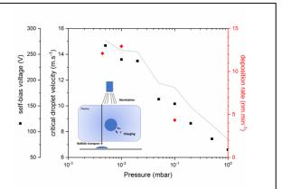
**Fig. 1.** Correlation between the self-bias voltage on the electrode (black squares), the critical droplet velocity to cross the sheath (black curve) and the thin film deposition rate for various argon pressure. The mechanisms considered are schematically described inset.
